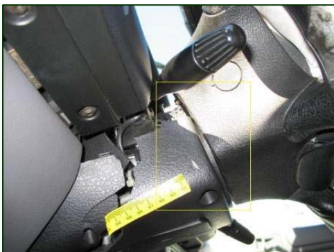
Figure 6. Steering wheel flange deformation.
