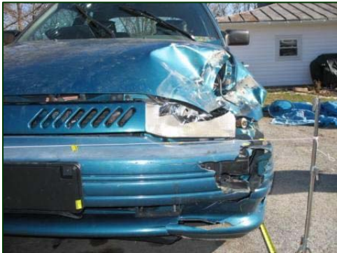
Figure 4. Direct contact damage on the frontal plane.
