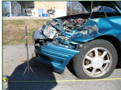
Figure 5. Extent of crush at the radiator support level.
