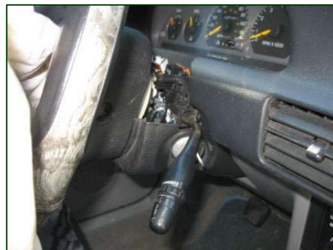
Figure 7. Wiper stalk deformed and fractured from column compression.
