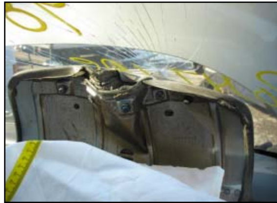
Figure 9. Steel backer panel deformation.
