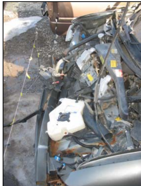
Figure 4. Left lateral view of the crush to upper radiator support.
