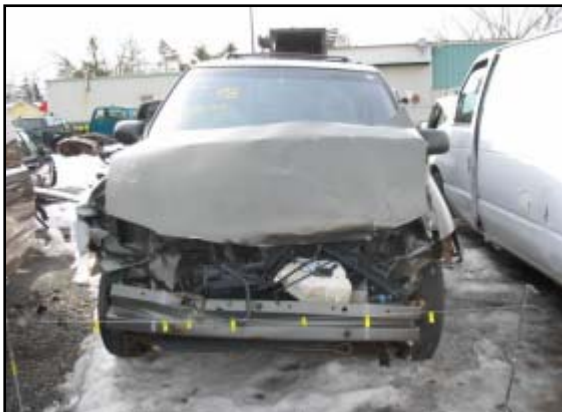
Figure 3. Frontal damage to the Pontiac.
