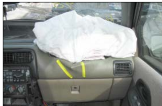
Figure 10. Damage to the instrument panel from the impeded deployment.
