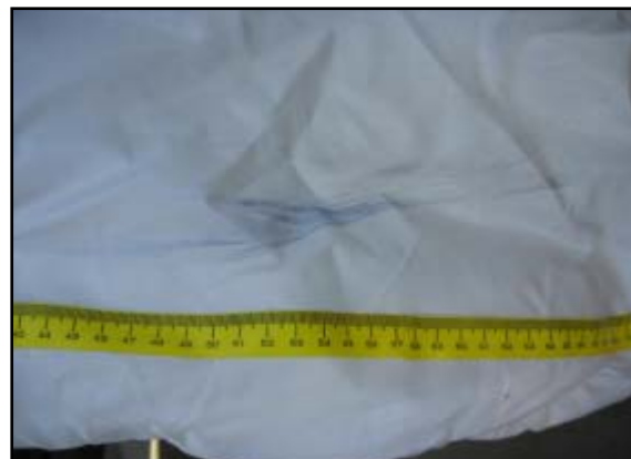
Figure 12. Blue fabric transfer on the right side pane.
