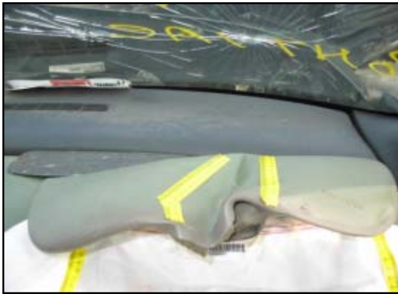
Figure 8. Deformed front right air bag module cover flap.
