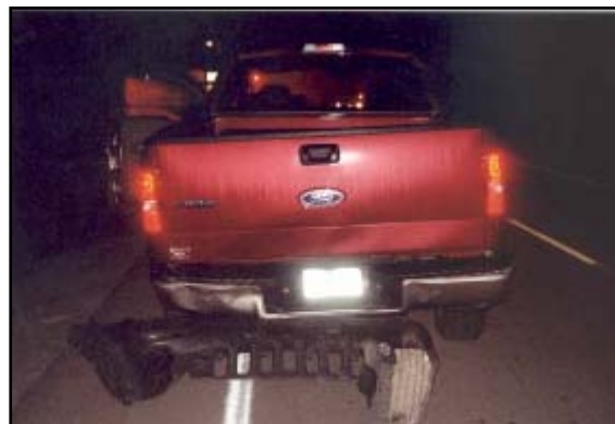
Figure 6. On-scene image of the resultant damage to the Ford.
