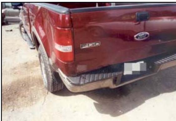
Figure 5. Rear plane damage to the Ford.
