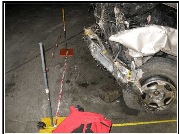
Figure 5. Left side view showing depth of crush at bumper level
