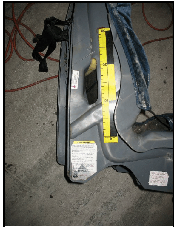
Figure 12. Load marks to booster seat anchor point on right
