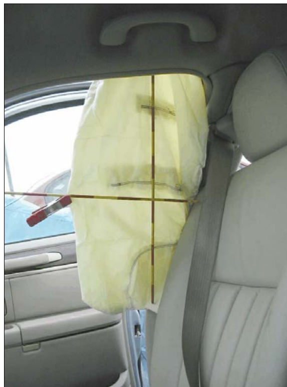
Figure 18: Lincoln’s front right passenger seat back-mounted side impact air bag, each increment on rods is 5 cm (2 in)
