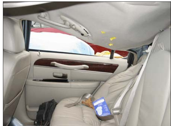
Figure 13: Overview of Lincoln's back right seat position and roof intrusion
