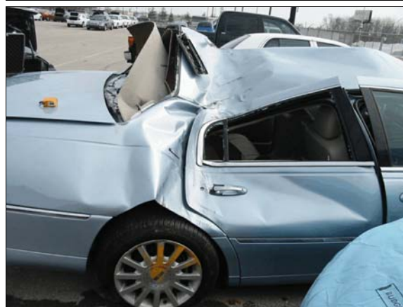
Figure 6: Damage to roof and right rear door due to impact with tree during rollover
