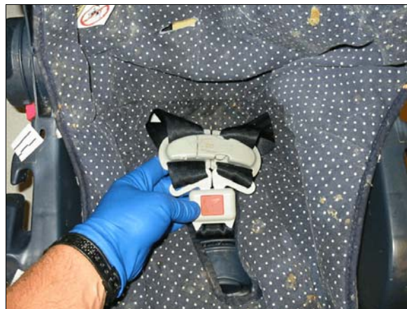
Figure 15: Shoulder harness straps routed through same slots in padded cover as lap belt straps, harness retainer clip positioned just above latch plates.
