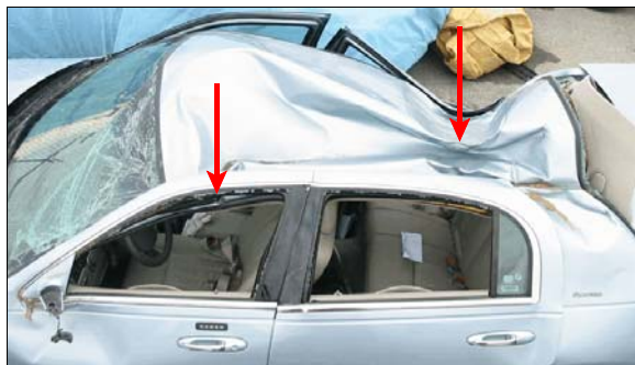
Figure 7: Left arrow shows location of maximum vertical and lateral crush due to the rollover; right arrow shows roof crush due to tree impact that occurred during rollover
