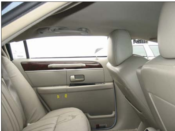
Figure 12: Overview of Lincoln's back left seat position and roof intrusion
