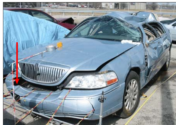
Figure 3: Overview of damage to front of Lincoln from fire hydrant impact (arrow) and rollover damage to roof
