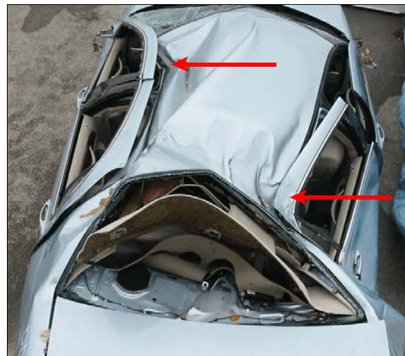
Figure 9: Left arrow shows location of maximum lateral crush to the roof due to rollover; right arrow shows crush from tree impact that occurred during rollover
