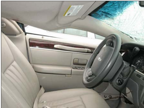
Figure 10: Overview of Lincoln driver's seat position and roof intrusion
