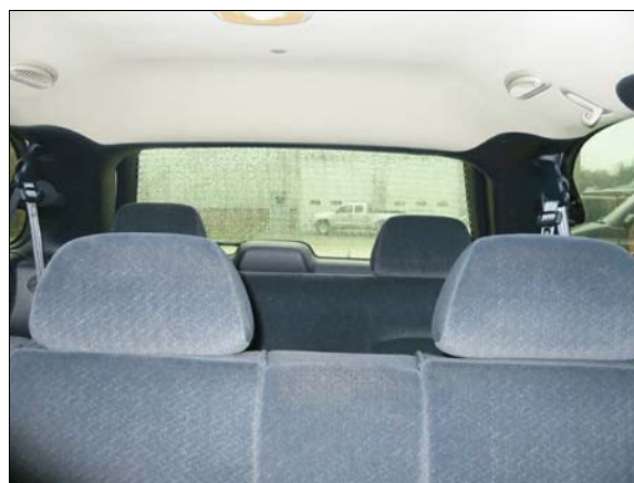
Figure 3: Driver's view out of backlight, note view obstructions by center high mounted stop lamp, head restraints and "D"-pillars
