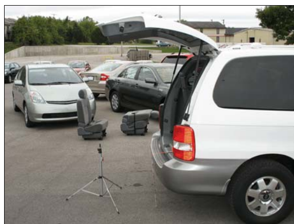
Figure 8: View of target set at location behind exemplar Kia where driver indicated he could first see it [55 centimeters (22 inches) back bumper to target] while looking over his right shoulder out of the open back hatch
