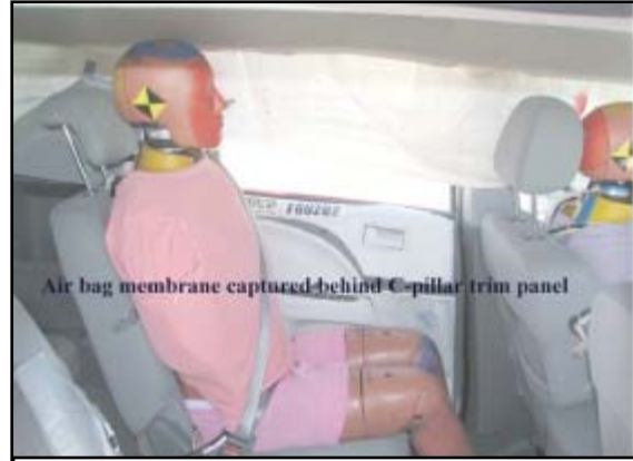
Figure 14. Post-test view of the deployed canopy air bag.
