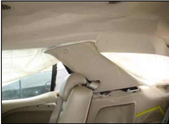
Figure 11. Canopy air bag membrane captured behind C-pillar trim panel.
