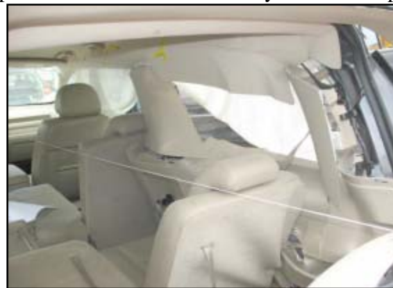
Figure 10. Deployed right canopy air bag.
