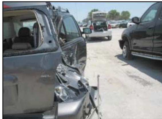
Figure 6. Longitudinal view of the crush.
