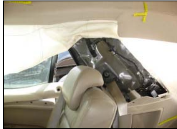
Figure 12. Air bag membrane with removed C-pillar trim panel. Note membrane was partially rolled similar to its un-deployed state.
