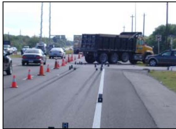
Figure 3. Freightliner's pre-impact skid marks.
