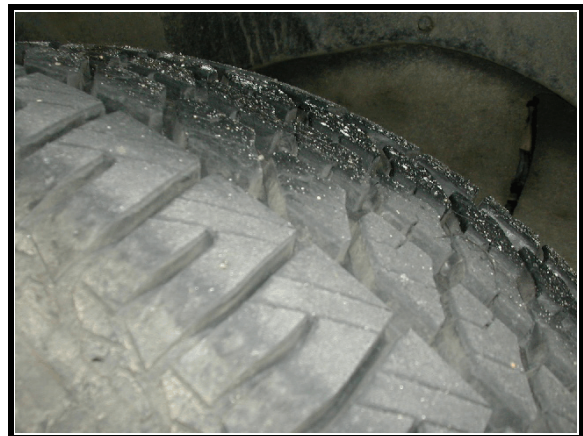
Figure 10. Oily substance found on right front tire tread
