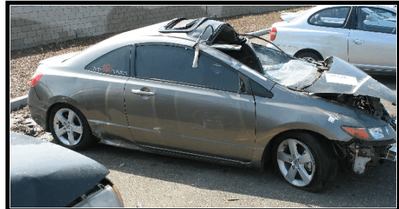
Figure 7. Right side damage (forward of rear tire)
