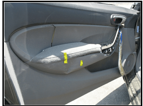
Figure 13. Occupant contact damage to door
