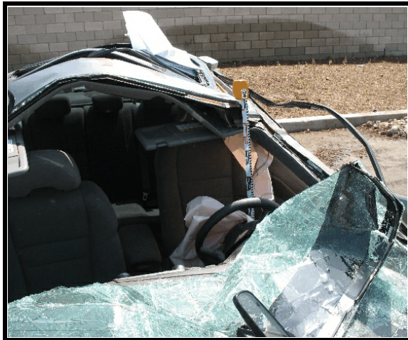
Figure 9. Exterior view of left side intrusion
