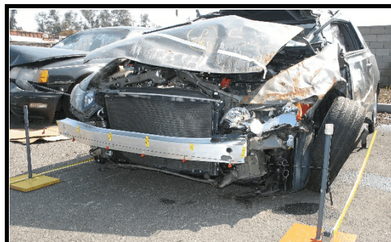
Figure 4. Front end damage, Honda Civic
