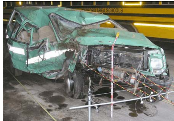
Figure 4: Damage to Jeep from impact with front of the Chevrolet; vertical scale in tenths of meter, each increment on measurement rods in 5 cm (2 in)
