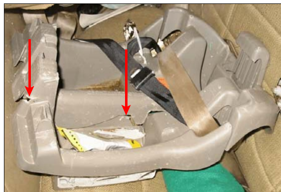
Figure 10: Infant seat base as found in Jeep's back center seat position, arrows show fractures in plastic
