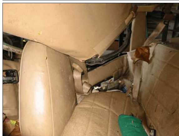
Figure 13: View from left showing Jeep's front right seat back pressed against back seat cushion and intrusion of roof into back right and back center seat positions
