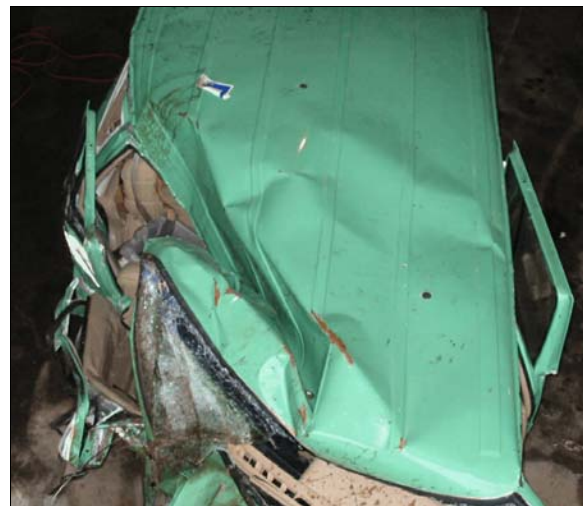
Figure 8: Induced damage folds to roof structure of Jeep due to front impact with the Chevrolet
