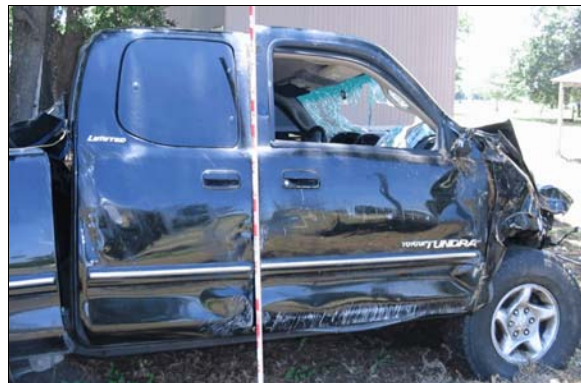
Figure 5: Pavement scratches to right side of Toyota's cab due to the rollover
