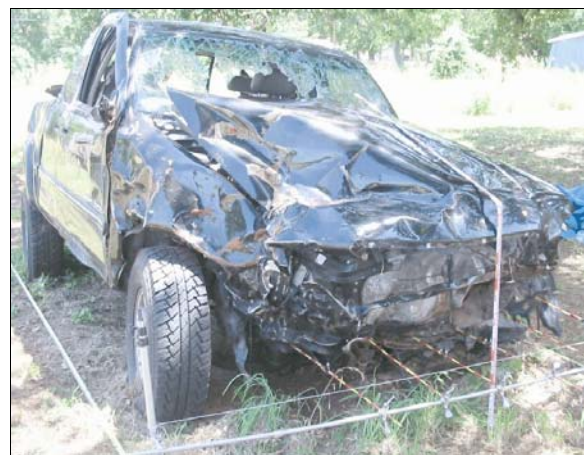
Figure 3: Damage to front of case vehicle due to impact with the Dodge, holed windshield is not related to crash
