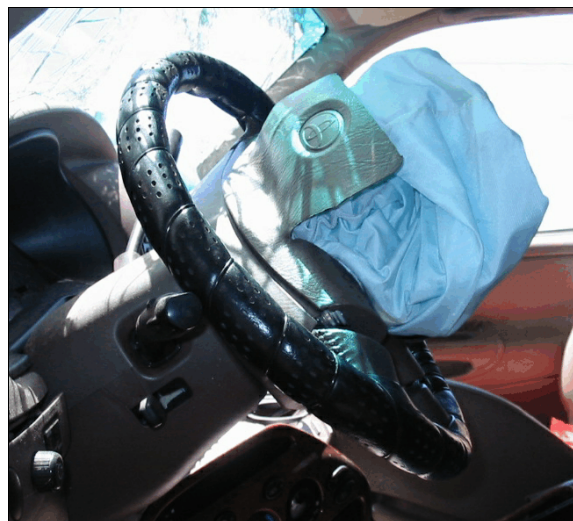
Figure 10: Left side view of deformation of top half of Toyota's steering wheel
