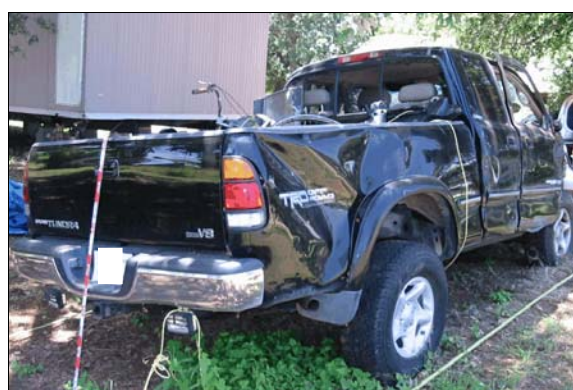
Figure 7: Overview of rollover damage to right side of Toyota and induced damage folds aft of right rear wheel due to rollover
