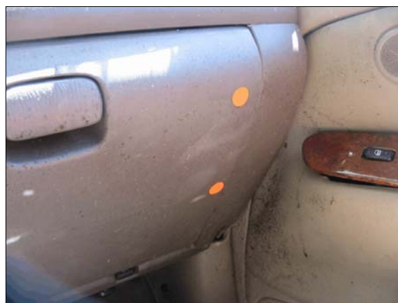
Figure 11: Orange dots show contact scuff on glove box door from front right passenger
