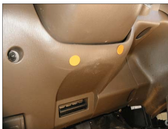
Figure 9: Occupant contact scuff on driver's knee bolster
