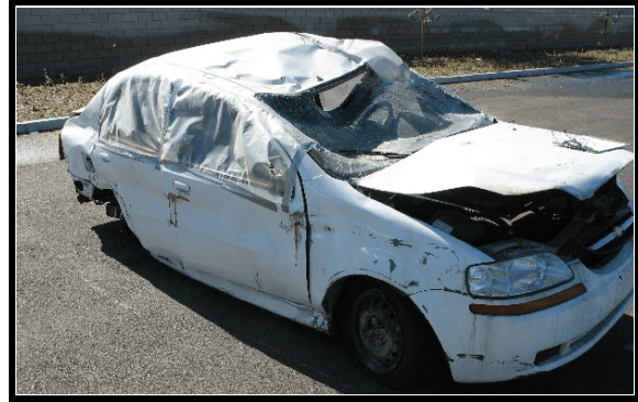
Figure 4. Damage from impact with barrier and rollover damage
