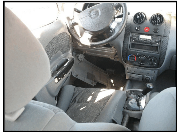
Figure 7. Left side intrusion
