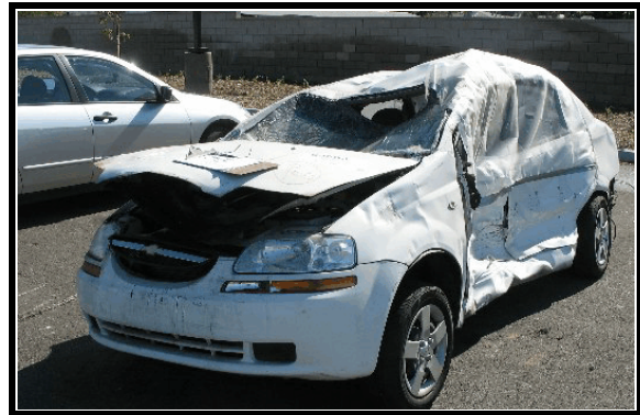
Figure 2. 2005 Chevrolet Aveo. Impact with other vehicle and rollover damage.
