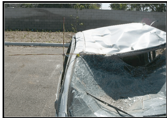
Figure 6. Maximum crush to roof from rollover
