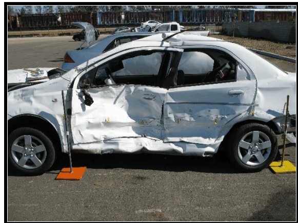
Figure 5. Damage from impact with Ford Focus
