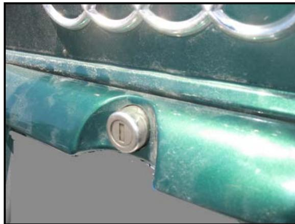
**Figure 5: Close-up view of the plunger trunk lock mechanism.**
