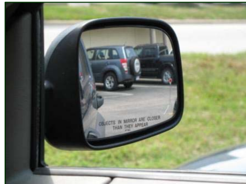
Figure 11. Right outside mirror visibility from the driver’s position.
