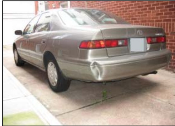
Figure 4. 1998 Toyota Camry. Note damage to the rear left bumper corner occurred while the vehicle was at an impound area.
