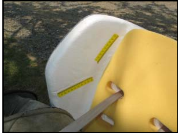
Figure 17: Fractured Styrofoam absorber.
