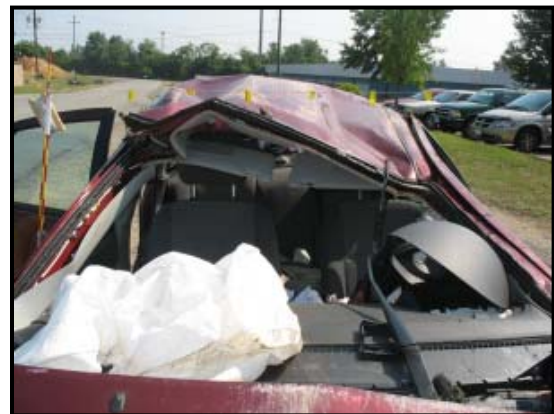
Figure 11: View of the maximum crush at the left A-pillar area.
