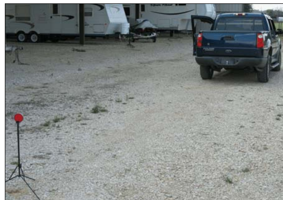
Figure 12: Closer view of target (tripod) where it became visible to Ford’s surrogate driver when looking over right shoulder—8.4 meters (27.6 feet) rearward of back of Ford
