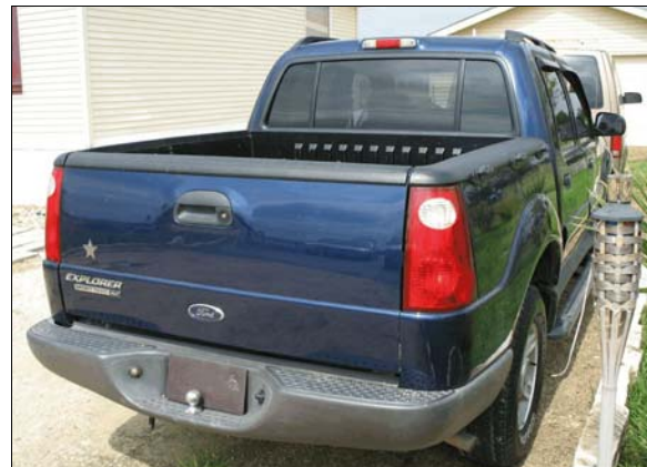
Figure 7: Ford's back viewed from right of back showing no apparent damage from contact with pedestrian
