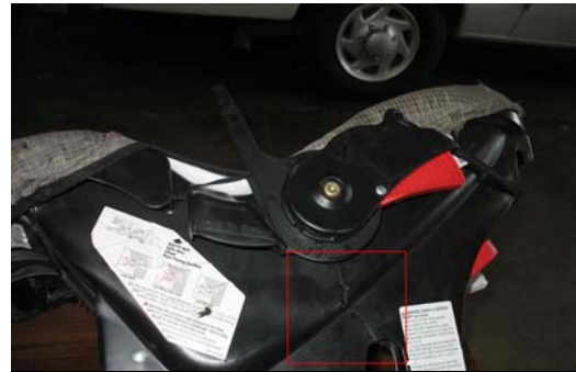
Figure 25 - Damage to the mid left aspect of the CSS.
