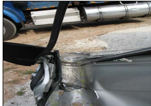
Figure 8 - Direct contact damage from the impact with the guard post.
