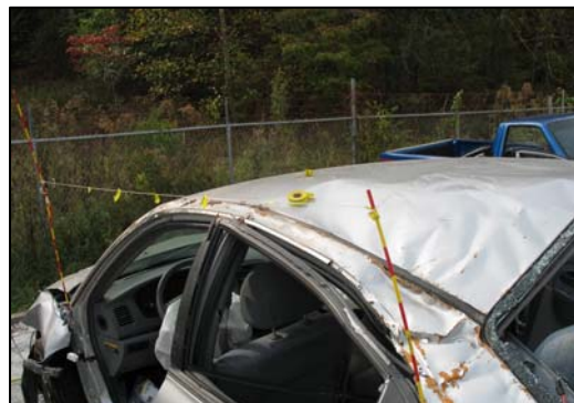
Figure 11 - Damaged roof and C-pillar of the Kia Optima.
