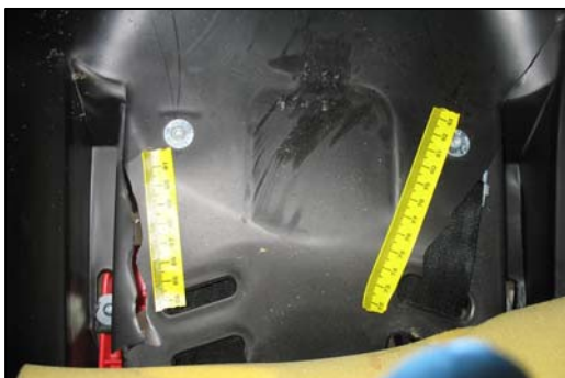
Figure 26 - Dual fractures to the back of the CSS.
