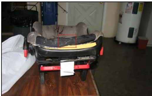
Figure 22 - Damage and paint transfers to the top of CSS.
