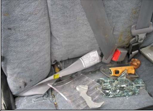
Figure 17 - Engaged right rear lap and shoulder belt.
