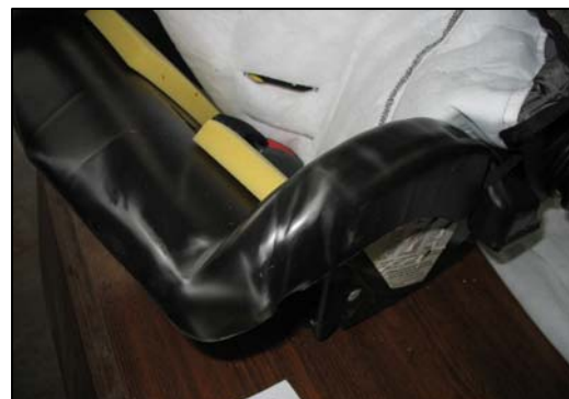
Figure 20 - Stress marks on lower left frontal aspect of the CSS shell.
