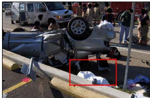
Figure 2 - The final rest position of the CSS (outlined) in relation to the Kia Optima.
