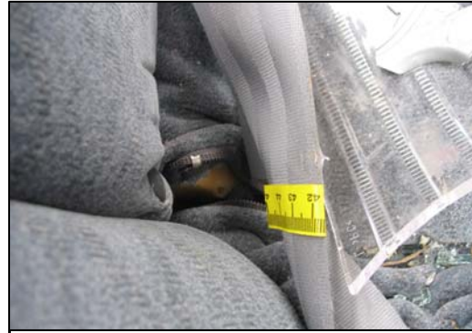
Figure 18 - Small tear in lap belt webbing.
