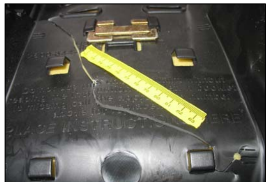
Figure 27 - Diagonally oriented fracture to the back of the CSS.
