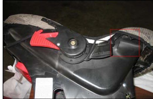
Figure 21 - Fractured right belt path.
