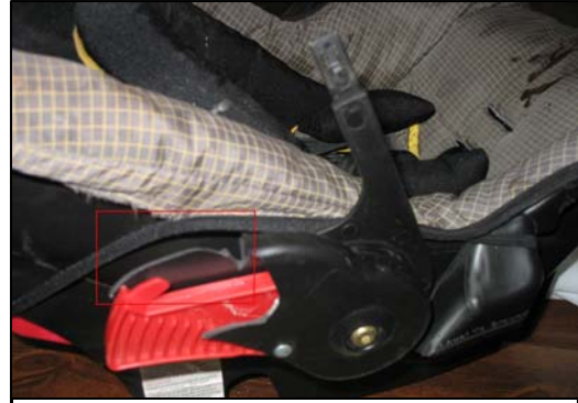
Figure 24 - Damage to the mid right side aspect of the CSS.
