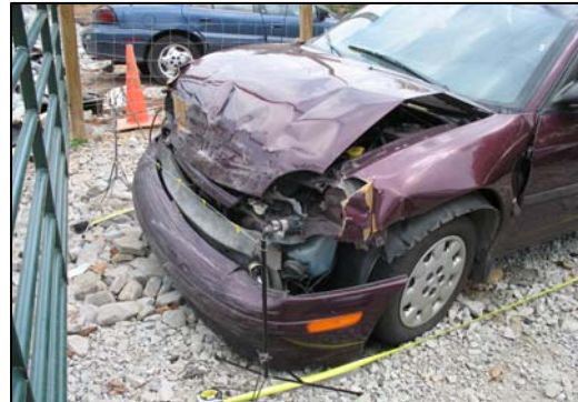
Figure 14 - Frontal damage to 1999 Dodge Neon.
