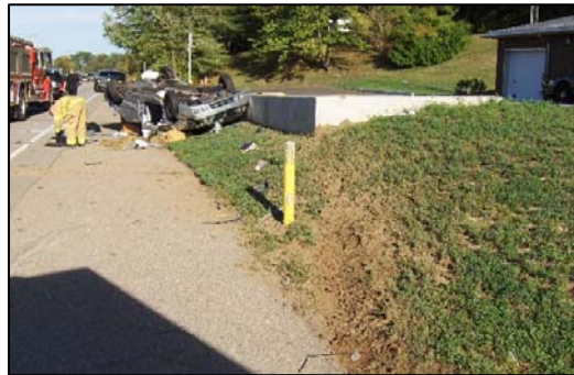
Figure 5 - Post-impact trajectory of the Kia, including the impacted guard post, retaining wall, and the area of final rest.
