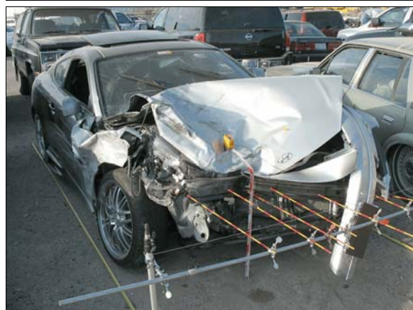
Figure 4: Hyundai's front damage from the impact with the back of the Chevrolet
