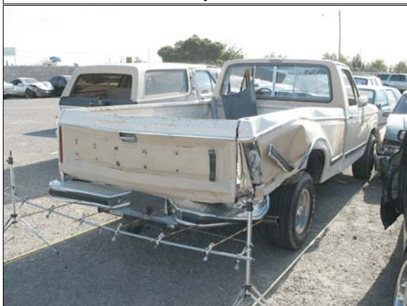
Figure 7: Damage to back of the Ford from the impact with the front of the Chevrolet
