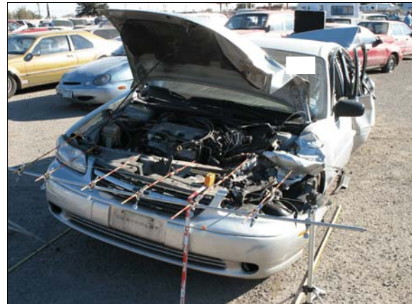
Figure 6: Damage to the front of the Chevrolet from impact with the back of the Ford
