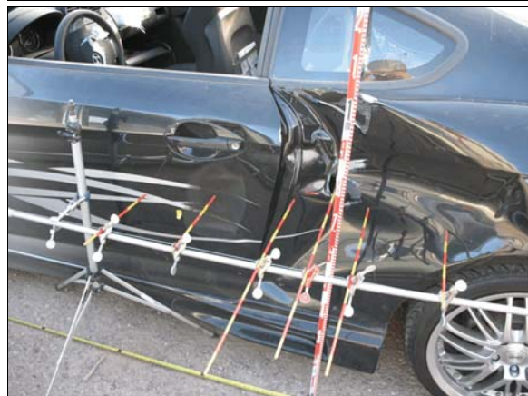
Figure 3: Hyundai's left side damage from the impact with the semitrailer
