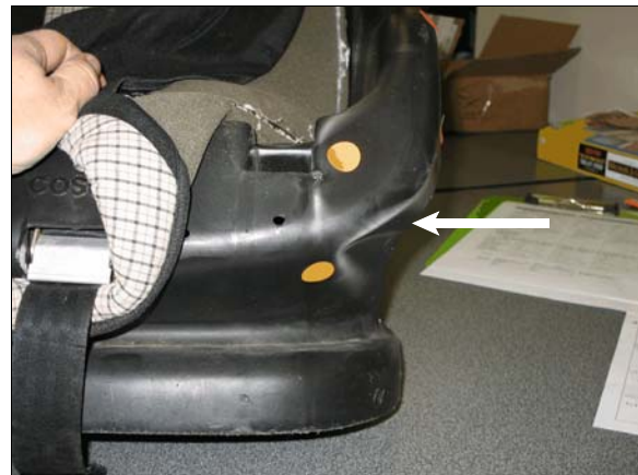
Figure 12: Deformation of second row left CSS (arrow)
