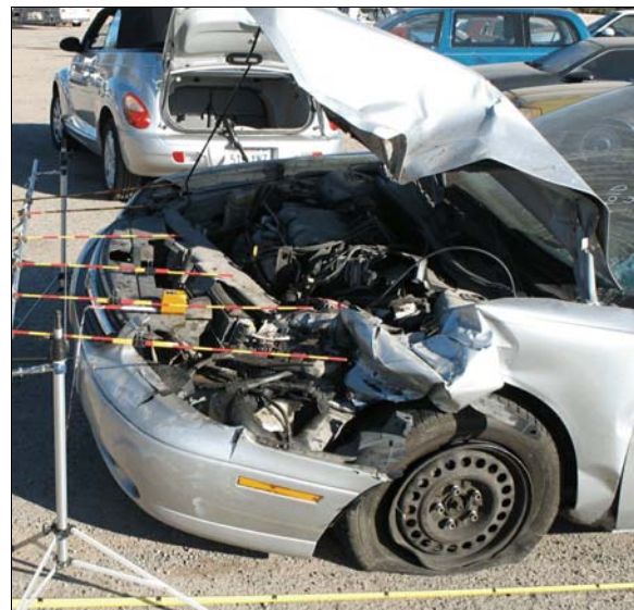
Figure 10: Left side view of the Chevrolet’s above bumper crush
