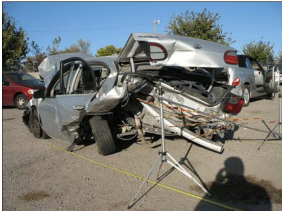
Figure 5: Damage to back of Chevrolet from impact with the front of the Hyundai
