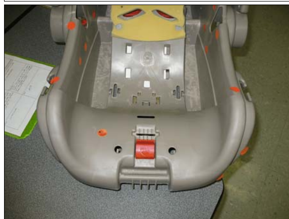
Figure 14: Orange dots show load marks in plastic shell of second row center CSS
