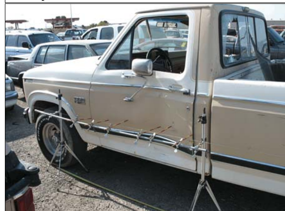
Figure 8 Damage to the Ford's left front door from impact with the Chevrolet's left quarter panel
