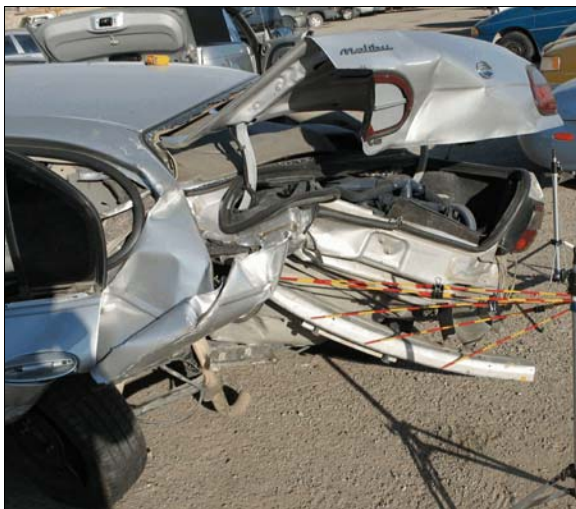
Figure 9: Left side view of the crush to the back of the Chevrolet
