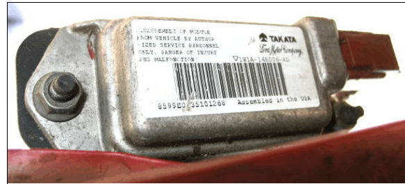
Figure 20: Mercury's impact sensor mounted at center of upper radiator support
