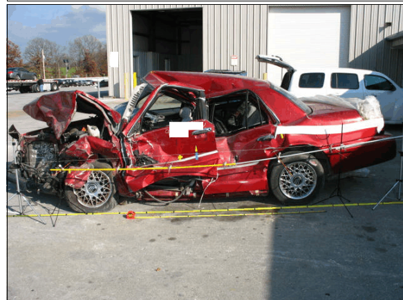
Figure 8: Damage to left side of Mercury due to impact with front of the International
