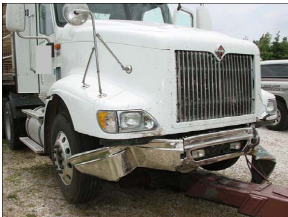
Figure 7: Police photo showing damage to front of International due to impact with left side of Mercury
