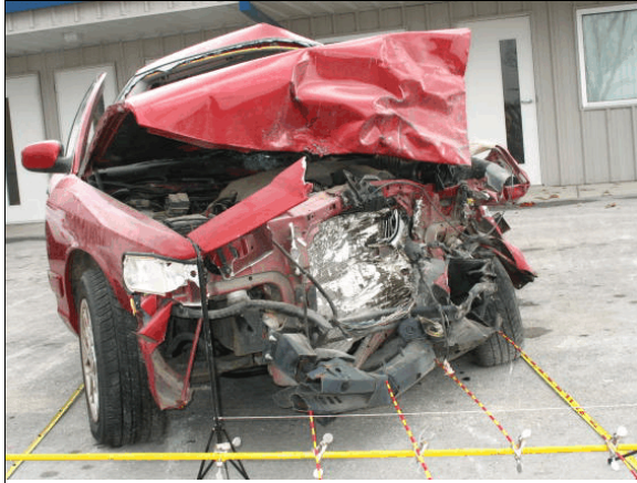
Figure 5: Overview of damage to front of Mercury from impact with front of the Lincoln
