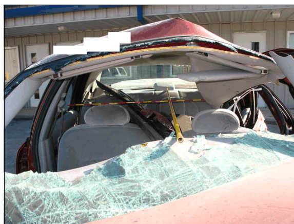
Figure 13: Left side intruding components into Mercury’s passenger compartment
