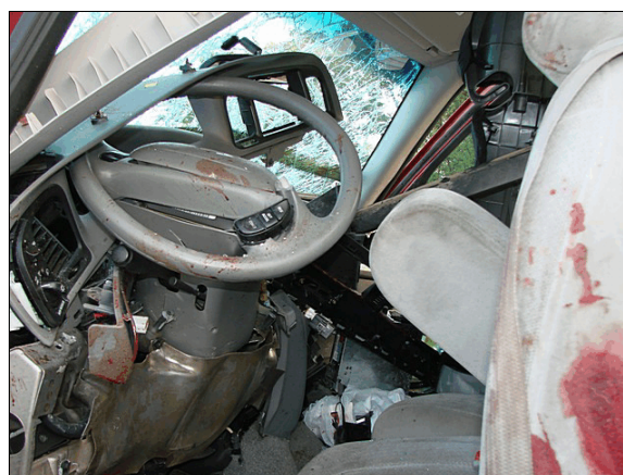
Figure 12: Police photo showing deformation to Mercury’s steering wheel and steering column
