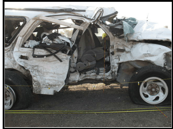
Figure 8. Subject vehicle, right side damage, middle
