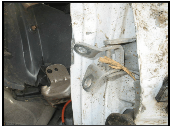
Figure 9. Upper hinge, first row right side door, subject vehicle
