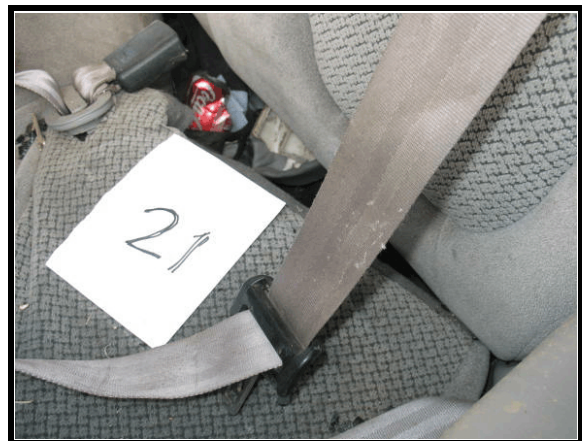
Figure 15. Second row left safety belt, showing evidence of occupant loading
