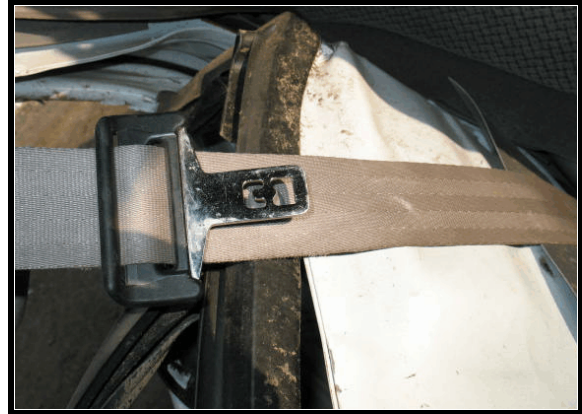
Figure 17. Second row right safety belt, showing evidence of occupant loading
