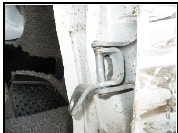
Figure 10. Lower hinge, first row right side door, subject vehicle
