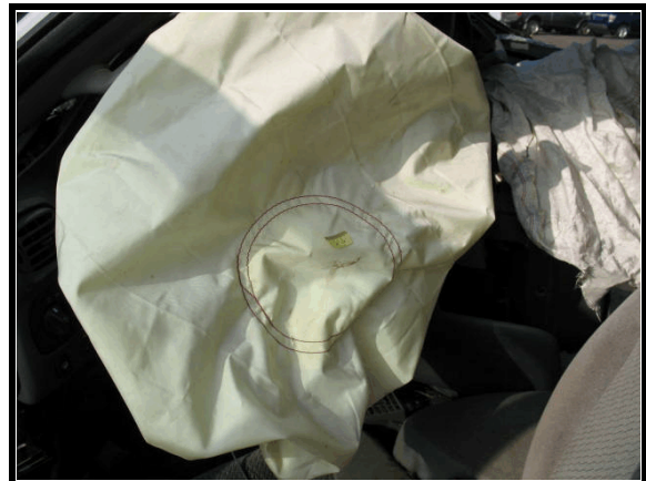
Figure 18. Driver air bag, showing suspected area of occupant contact
