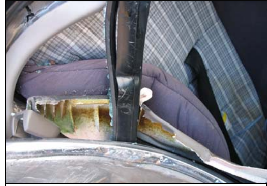
Figure 13 - Intruded door panel and quarter window frame against CSS shell.
