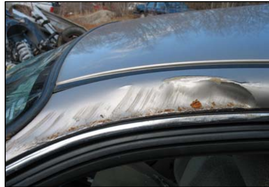
Figure 6 - Damage to left roof side rail.
