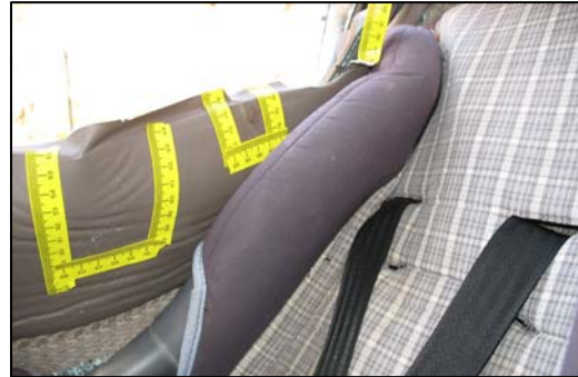
Figure 7 - Areas of probable occupant contact.
