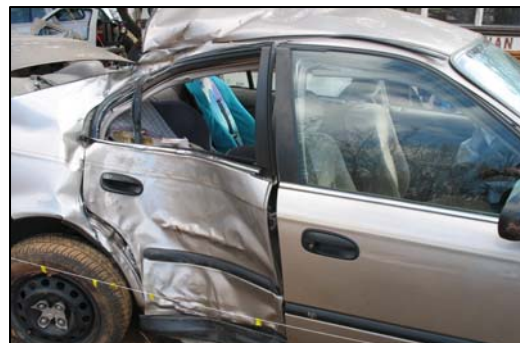
Figure 5 - Damage to right rear door area.
