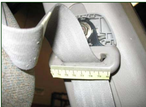
Figure 15. Frictional abrasion on belt webbing and D-ring.
