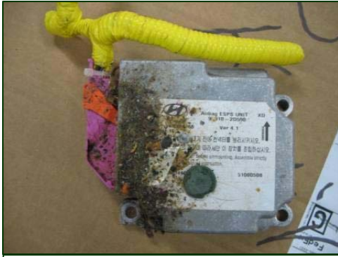
Figure 11. Removed ACM and pin connector.
