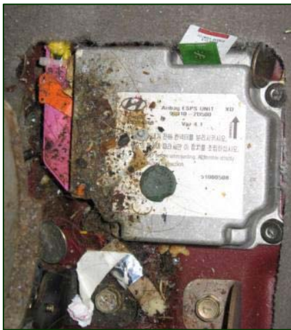
Figure 9. ACM and connector as found in vehicle.
