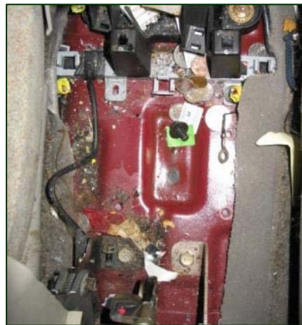
Figure 10. Condition of console floor with ACM removed.
