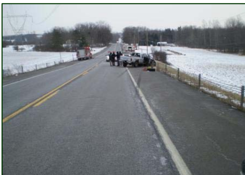
Figure 3. Trajectory of the Toyota and the pre-crash skid marks.
