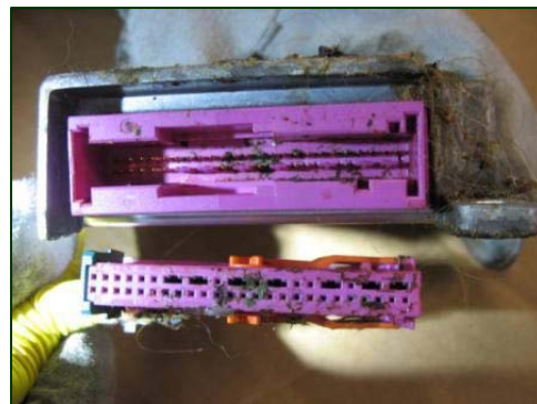
Figure 14. Corrosion at mid point of connector and pins.
