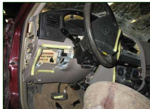
Figure 16. Driver loading of the steering assembly and the mid instrument panel.
