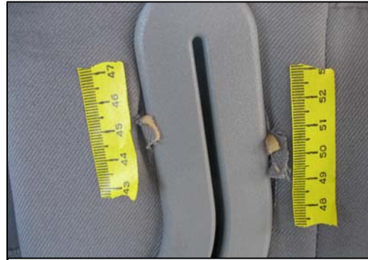
Figure 7 - Damaged guide path for second row center shoulder restraint.
