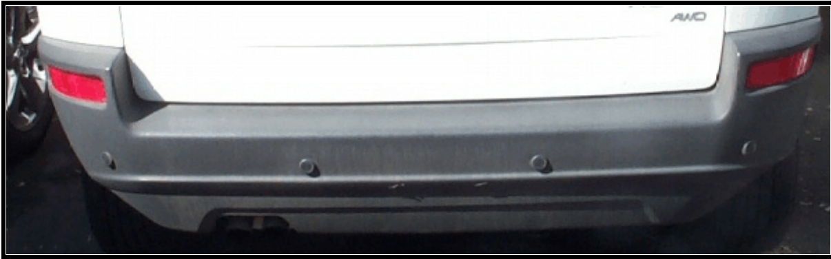
Figure 5. Rear parking assistance system sensors (subject vehicle)
