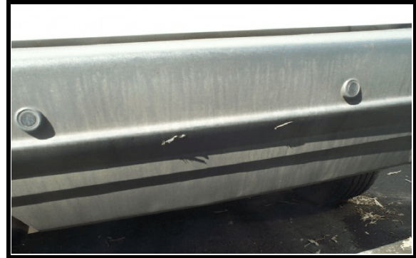
Figure 12. Gouges located on rear bumper
