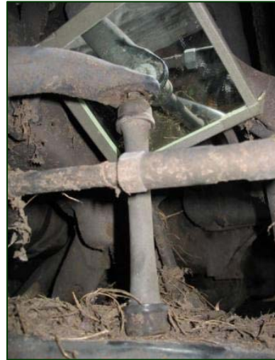
Figure 15. Left front stabilizer link with top bushing absent.
