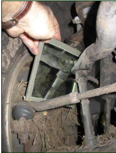
Figure 14. Right front stabilizer link with standoff bushings intact.
