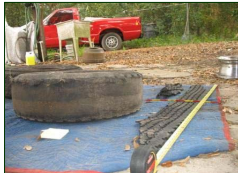
Figure 12. Separated tire tread and the tire ply surface.
