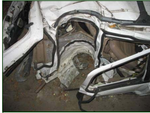
Figure 9. Overhead view of the lateral impact damage to the right rear quarter panel.
