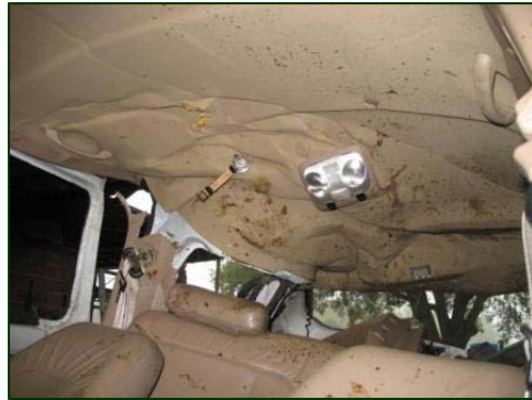
Figure 13. Intrusion and occupant contact points within the interior of the Explorer.
