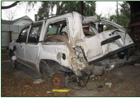
Figure 7. Event #1 damage to the back left corner area.
