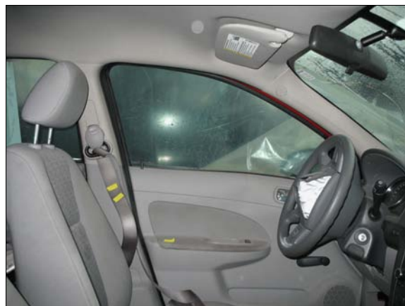
Figure 7: Chevrolet’s driver seating area showing deployed driver air bag, steering wheel, greenhouse, driver’s safety belt—with evidence of loading, and contact on interior door surface
