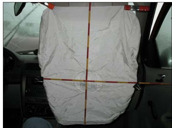
Figure 13: Chevrolet's deployed front right passenger air bag showing no occupant contact evidence
