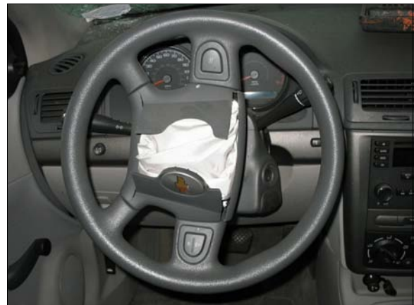
Figure 10: Chevrolet’s steering wheel with driver air bag module and flaps; steering wheel rotated clockwise approximately 90 degrees
