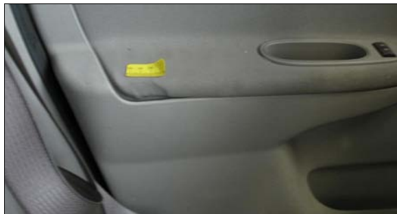
Figure 8: Close-up of dent in arm rest of Chevrolet’s driver door from driver contact
