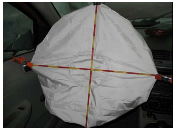
Figure 11: Chevrolet’s deployed driver air bag showing no obvious evidence of occupant contact
