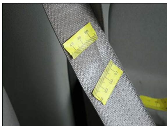
Figure 9: Load mark on Chevrolet’s driver shoulder belt webbing
