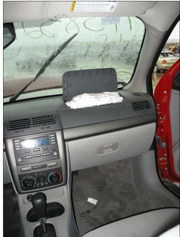
Figure 12: Chevrolet's front right seating area showing deployed front right air bag, center and right instrument panels, center console, and greenhouse area; no occupant contacts evident
