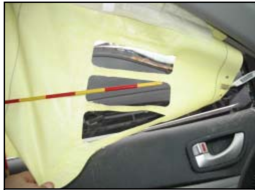
Figure 13. Cut outs on forward aspect of the curtain air bag.
