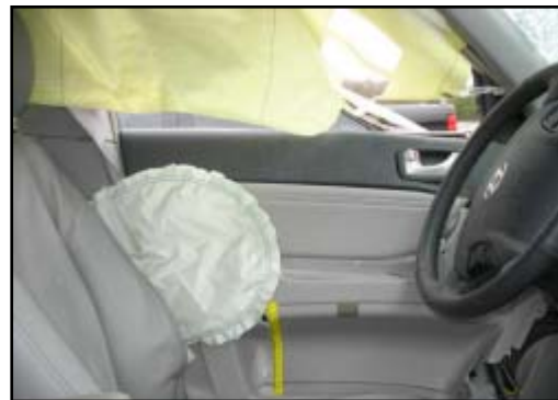
Figure 11. Deployed left seatback mounted side impact air bag.
