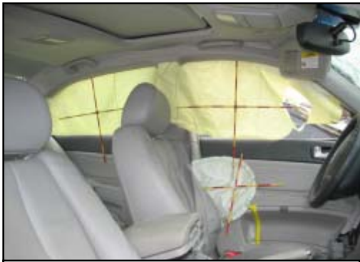
Figure 12. Deployed left side curtain air bag.
