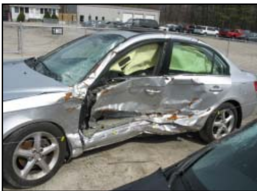
Figure 4. Residual damage to the left side of the Hyundai Sonata.
