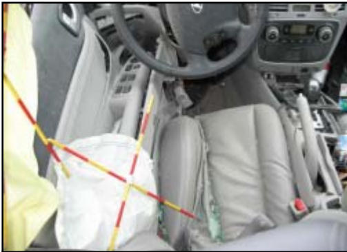
Figure 7. Lateral intrusion into the driver's position.
