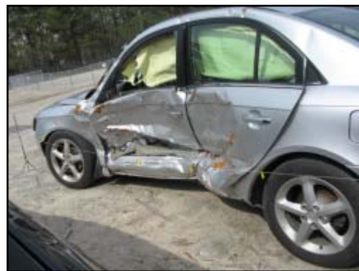
Figure 5. Oblique view of the left side crush.
