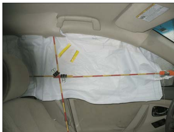
Figure 7: Yellow tape shows makeup smear from driver contact on left side curtain air bag
