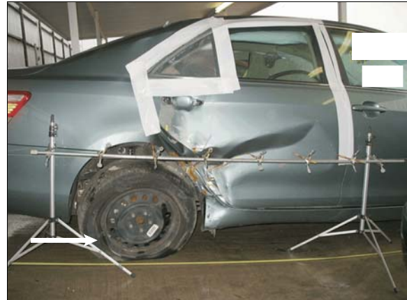
Figure 6: Arrow shows damage to right rear wheel from curb impact; damage to right rear door from impact with the traffic signal pole
