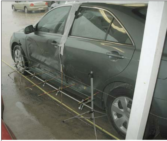
Figure 5: Damage to left side of Toyota from impact with front of Mitsubishi
