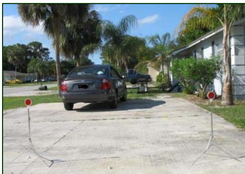
Figure 9. Lateral cone of visibility through the right outside mirror.
