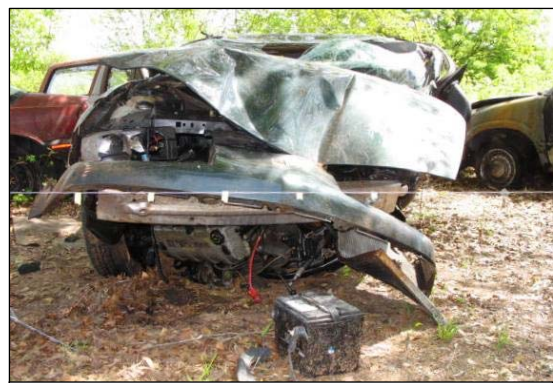
Figure 6: Frontal damage to the Saturn.
