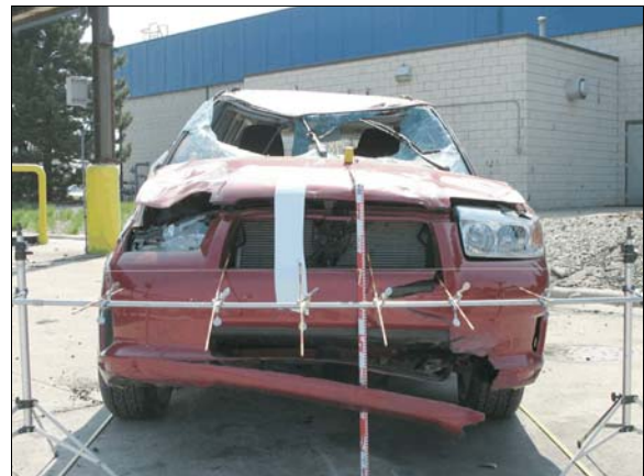
Figure 4: Damage to front of Subaru from impact with the culvert; scale numbers in tenths of meter
