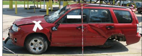
Figure 8: Damage to the left side from the rollover
