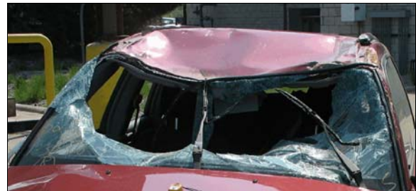
Figure 10: Crush to the windshield header and roof from the rollover
