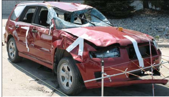
Figure 7: Front right view of the front damage and damage from the rollover
