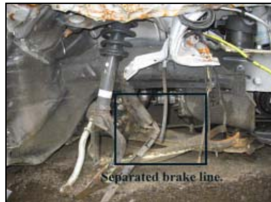
Figure 6. Separated right front brake line.
