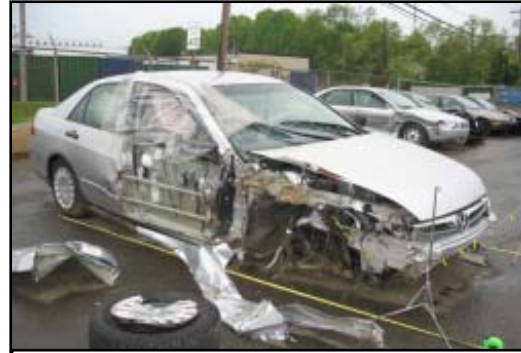
Figure 5. Damage to the right side of the Honda.
