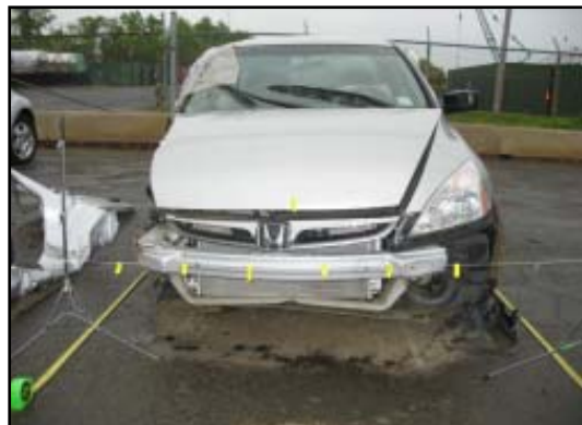
Figure 4. Resultant front damage.
