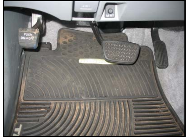
Figure 10: Rubber Mat displaced to its most forward position.
