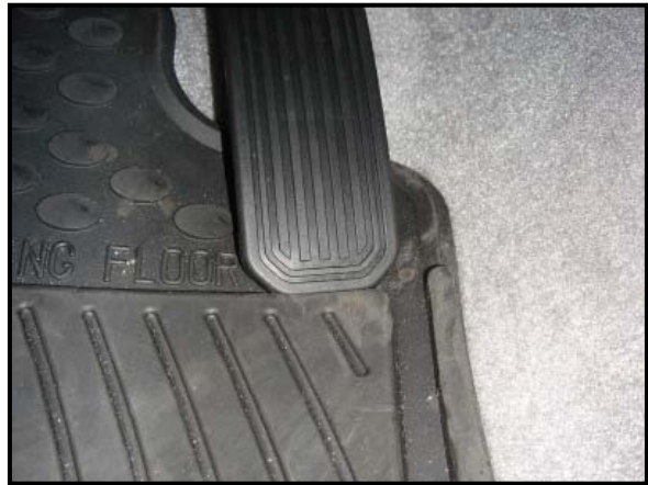
Figure 13: Close-up view of the entrapped accelerator pedal in Figure 12.
