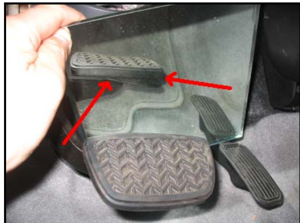
Figure 7: Displaced brake pedal pad.
