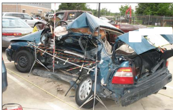
Figure 4: Damage to left side of 1994 Honda from impact with front of 2007 Honda
