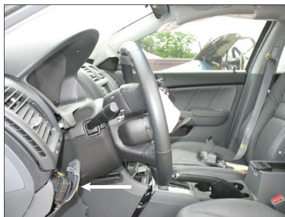
Figure 8: Left side view of deformation on the steering wheel and left lower instrument panel (arrow) due to driver loading
