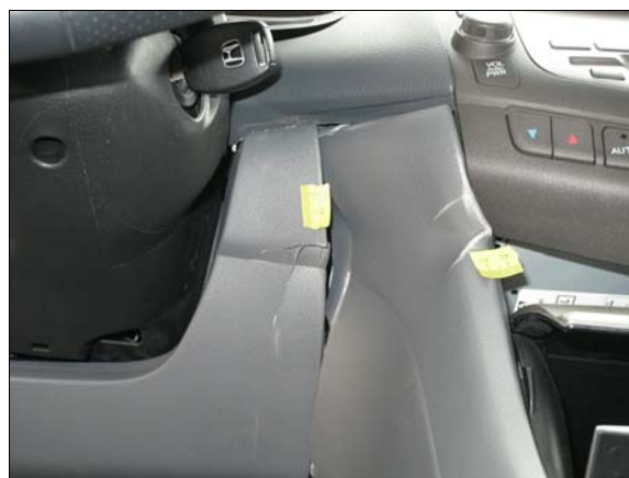
Figure 9: Deformation of the center lower instrument panel due to loading by the driver’s right knee
