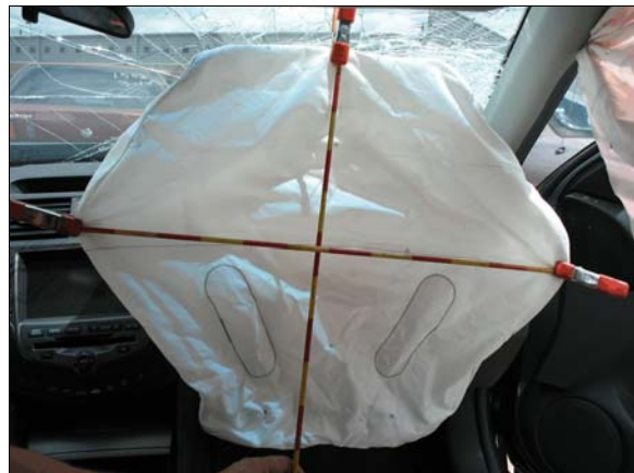
Figure 11: Front right passenger's deployed air bag
