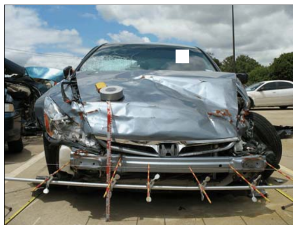
Figure 3: Damage to front of 2007 Honda from impact with left side of 1994 Honda
