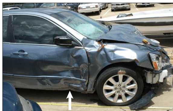
Figure 5: Damage to right fender and right front door of the 2007 Honda from impact with 1994 Honda left quarter panel; arrow shows overlapping damage from bus stop sign impact
