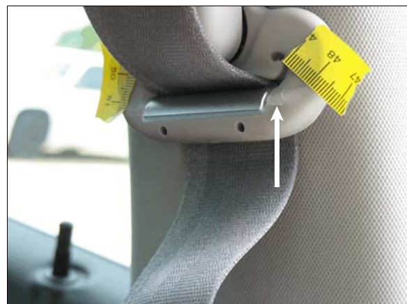
Figure 14: Arrow shows load abrasion on plastic of driver's D-ring
