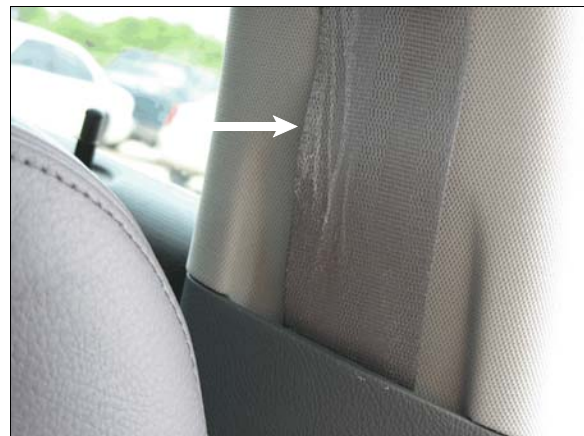
Figure 15: Load abrasions on driver's seat belt
