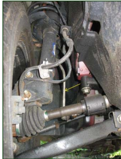
Figure 12. Deformed right front stabilizer link of the case vehicle.
