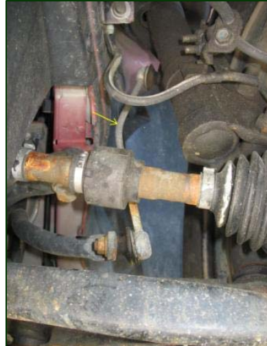
Figure 10. Deformed left front stabilizer link of the case vehicle.
