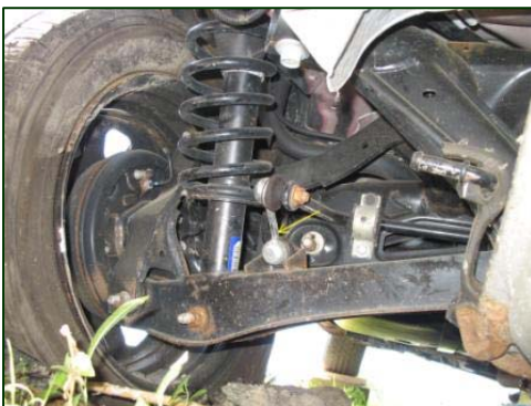
Figure 15. Deformed left rear stabilizer link of the 2007 Dodge Caliber.
