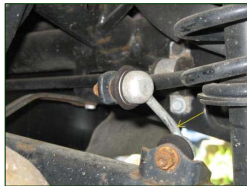
Figure 16. Deformed right rear stabilizer link of the 2007 Dodge Caliber.
