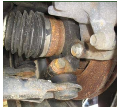
Figure 13. Intact lower left ball joint and outer tie rod of the 2007 Dodge Caliber.
