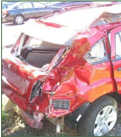
Figure 7. Right D-pillar area damage.
