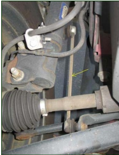
Figure 11. Right front stabilizer link of an exemplar vehicle.
