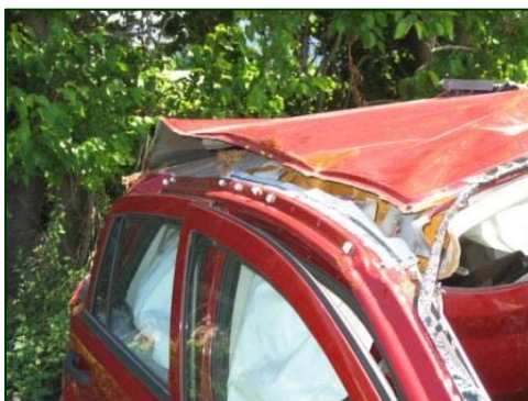
Figure 5. Separated roof panel.
