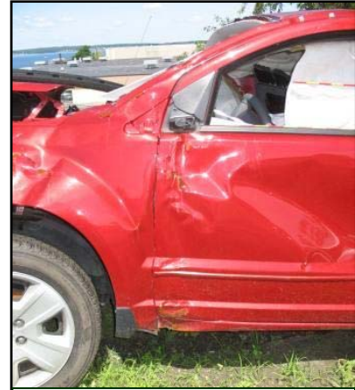
Figure 3. Delineator impact to the left front door.
