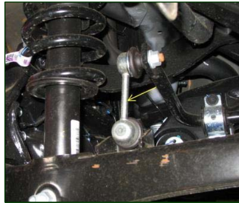
Figure 14. Left rear stabilizer link of an exemplar vehicle.
