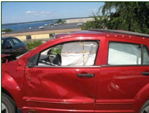
Figure 17. Exterior view of the deployed left IC air bag.
