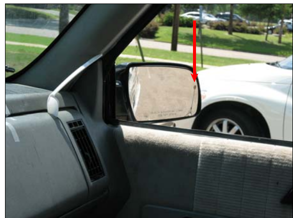
Figure 10: View through right side view mirror from the driver's seat, arrow shows target where it begins to go out of the mirror's lateral field of view
