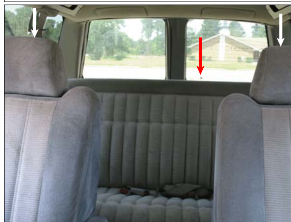
Figure 7: View out of backlight from driver's seat; arrows show target and second row captain's chairs
