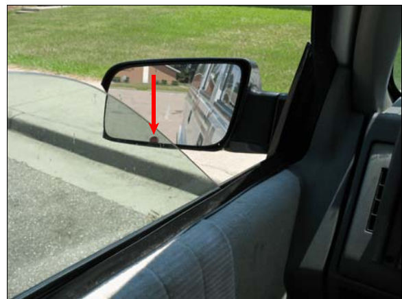
Figure 9: View through left side view mirror from driver's seat; arrow shows target where it begins to go out of the mirror's bottom field of view
