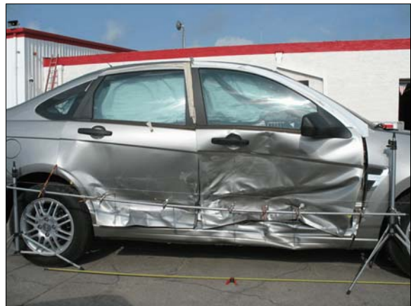
Figure 5: Damage to Ford's right side from impact with the Toyota
