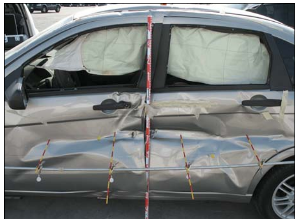
Figure 6: Damage to the Ford's left side from impact with the Chevrolet
