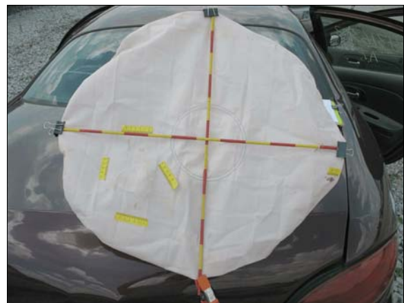
Figure 9: The driver's deployed air bag; yellow tape shows body fluid deposit on left
