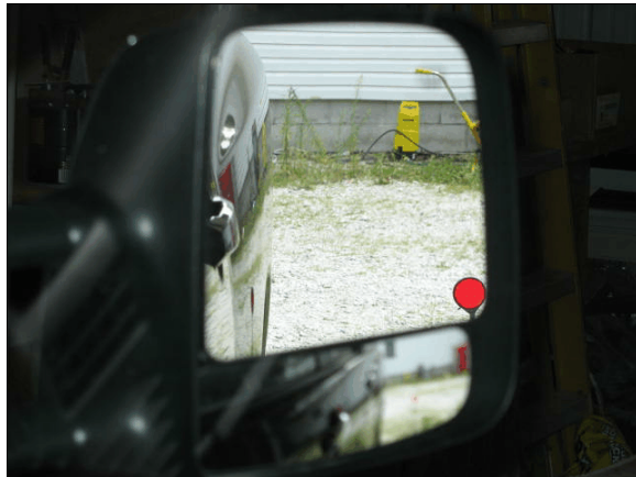
Figure 10: Close view through right side view mirror from driver's seat; target in location where it began to go out of mirror's lateral field of view
