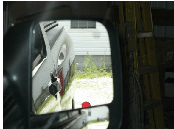
Figure 9: Close view through right side view mirror from driver's seat; target in location where driver could first see it as it was moved rearward along right side of vehicle
