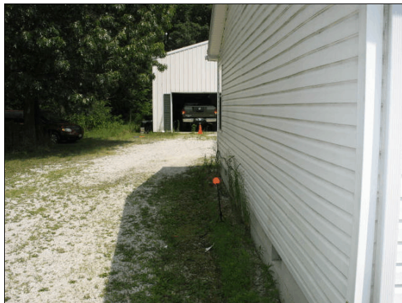
Figure 12: Location of target where driver could first see it while looking through rearview mirror; distance from back bumper to target was 17.6 meters (57.7 feet)
