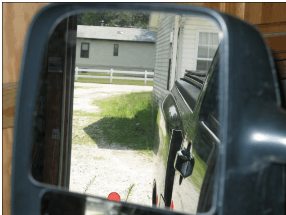
Figure 8: Close view through left side view mirror from driver's seat; target where driver could first see it as moved rearward along left side of vehicle
