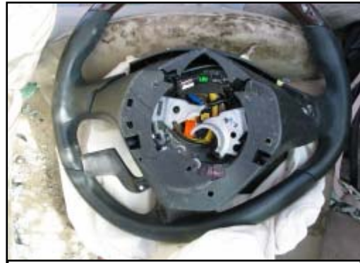
Figure 8. Fractured steering wheel flange.
