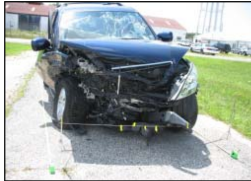
Figure 9. Resultant frontal damage to the Lexus.
