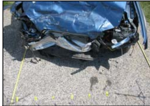
Figure 6. Overhead view of the resultant crush to the Subaru.
