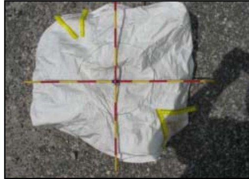
Figure 12. Body fluid transfers on the driver's air bag membrane.
