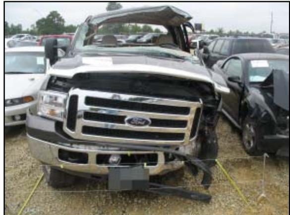
**Figure 4: Overall view of the frontal damage**
