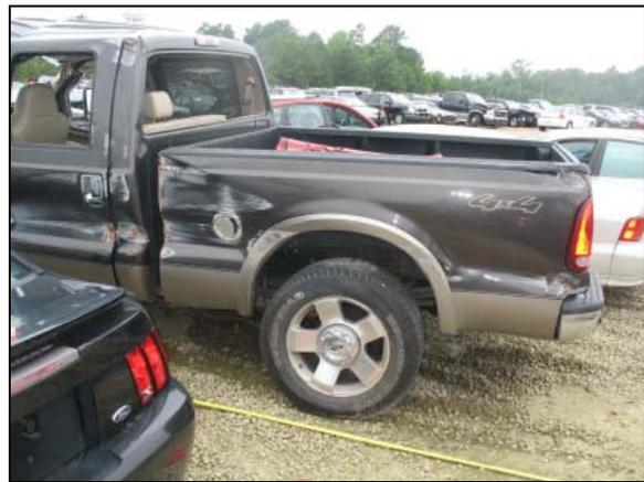
Figure 6: View of the Ford's left side damage.
