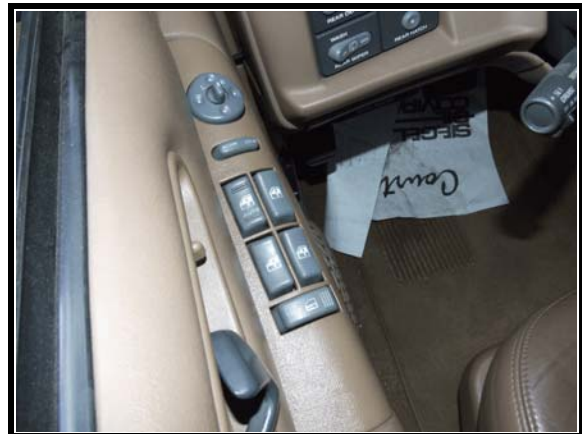
Figure 7. Driver's power switch control
