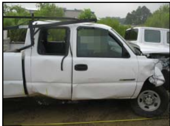
Figure 6: Right sill damage from the utility pole impact.
