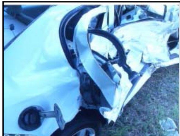
Figure 8: View of the damage to the right plane of the Chevrolet Cobalt. Insurance company image.
