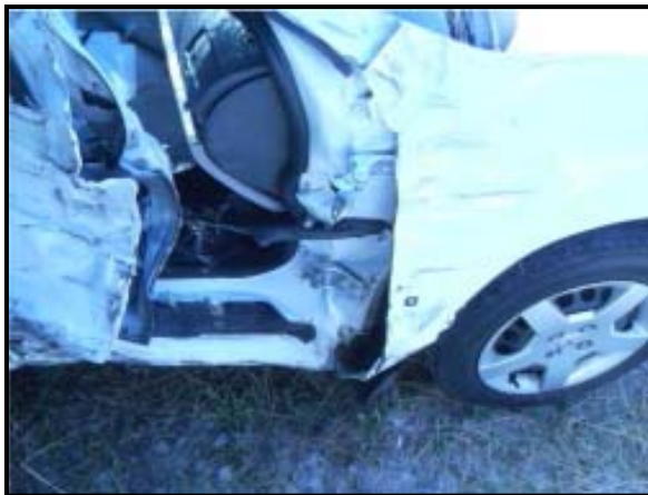
Figure 7: Right view of the damage at the A-pillar of the Chevrolet Cobalt. Image supplied by the vehicle's insurance company.
