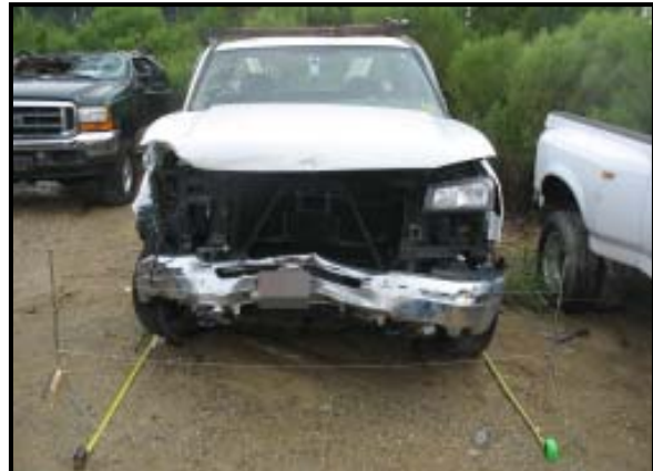
Figure 4: Residual front damage from the impact with the Chevrolet Cobalt.
