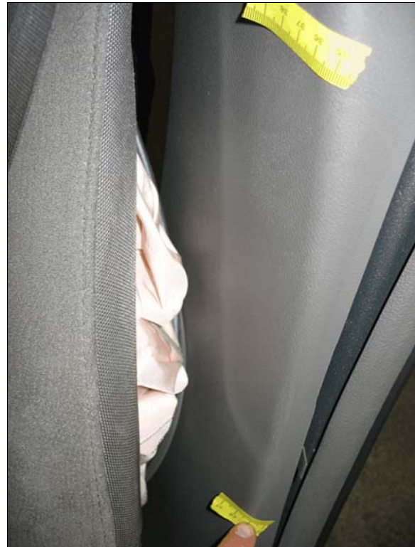
Figure 12: Locations of driver's seat back-mounted side impact air bag; yellow tape highlights light abrasions on B-pillar from the deployment
