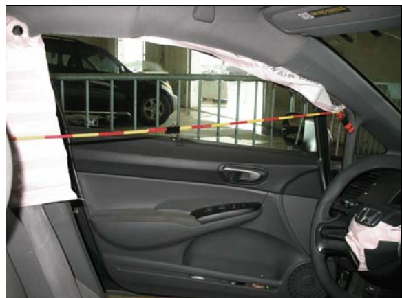
Figure 10: Front portion of left side curtain air bag had been cut away by emergency personnel
