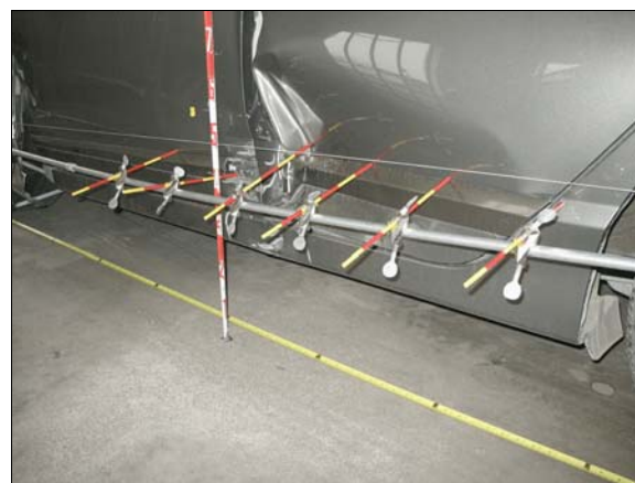
Figure 7: Damage on the left side plane from the impact with the Buick's right rear corner
