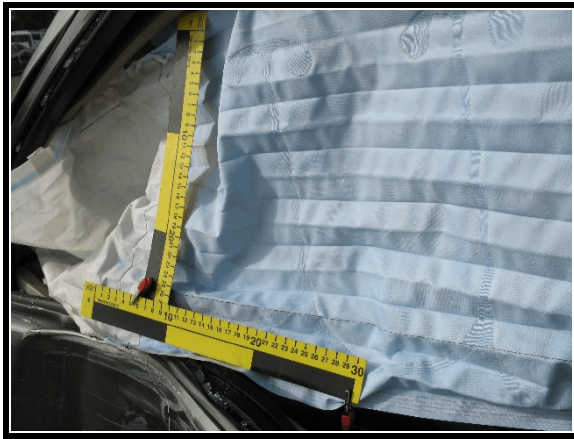
Figure 10. Scuff located on outboard side of left side curtain air bag
