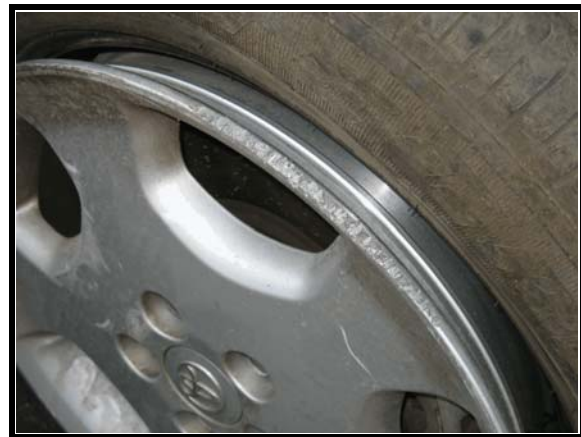
Figure 5. Damage to right front rim
