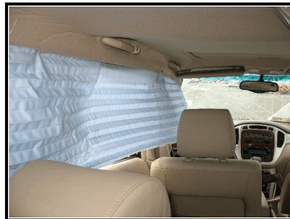
Figure 9. Side curtain air bag
