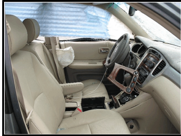
Figure 11. Side curtain air bag and seat-mounted side air bag
