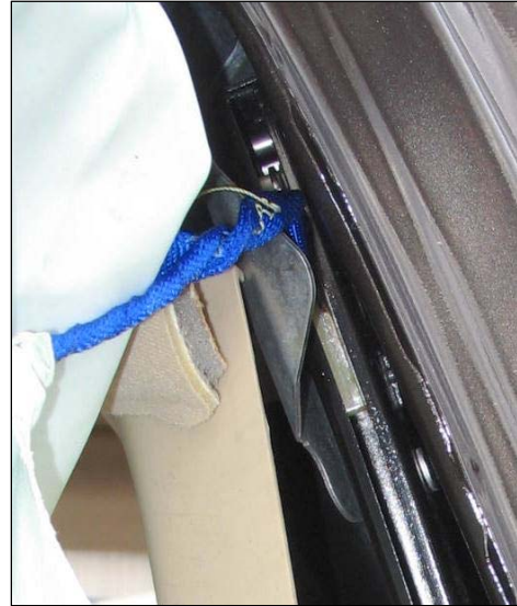
Figure 12: Rear tether of left IC snagged on metal bracket.
