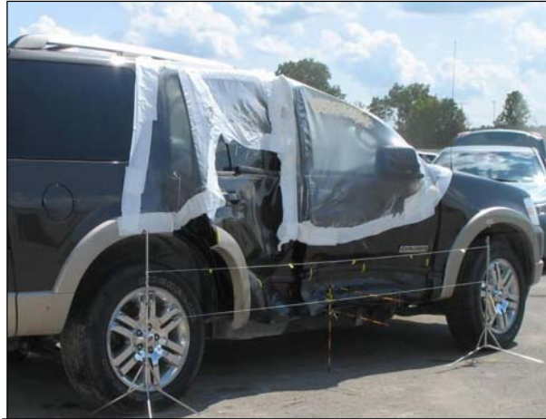
Figure 5: Side impact damage to the Ford.
