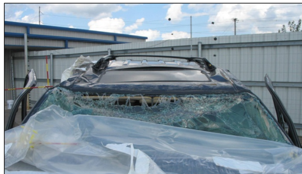
Figure 6: Rollover damage to the Ford's roof.
