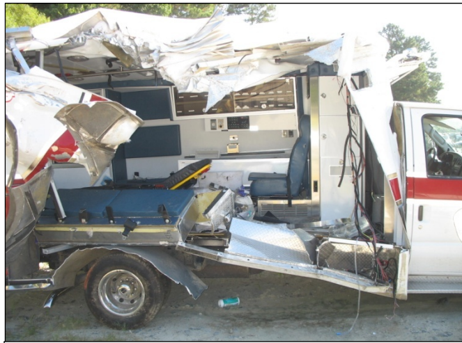
Figure 11: Integrity loss to right side of ambulance module.
