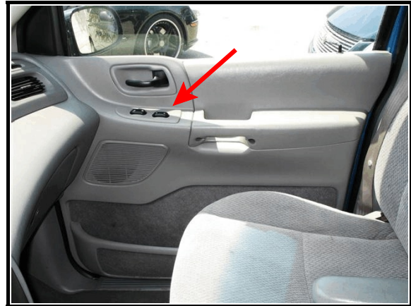
Figure 1. 2001 Ford Windstar exemplar vehicle showing power window switch location
