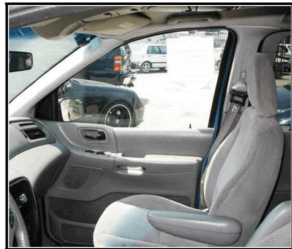
Figure 2. 2001 Ford Windstar exemplar vehicle showing window used for closing force test
