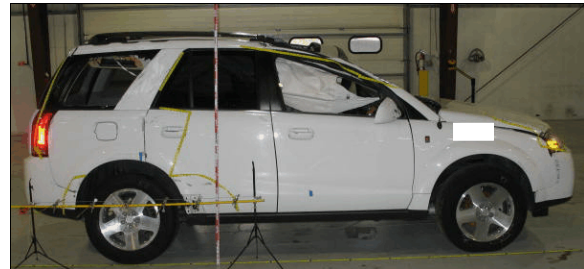
Figure 7: Yellow tape above the level of the right rear wheel outlines the damage from the rollover
