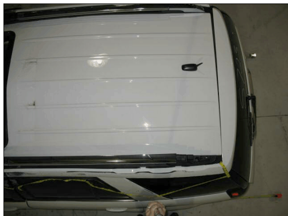
Figure 10: Damage on left roof side rail and luggage rack from the rollover
