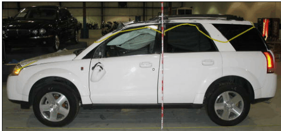
Figure 6: Left side of Saturn; yellow tape outlines damage from the rollover
